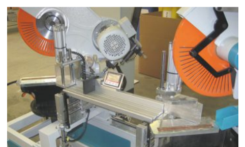
Both saw units for the left and right cuts, parallel and exactly to the specified length dimension are automatically adjusted at the push of a button on the control panel.
