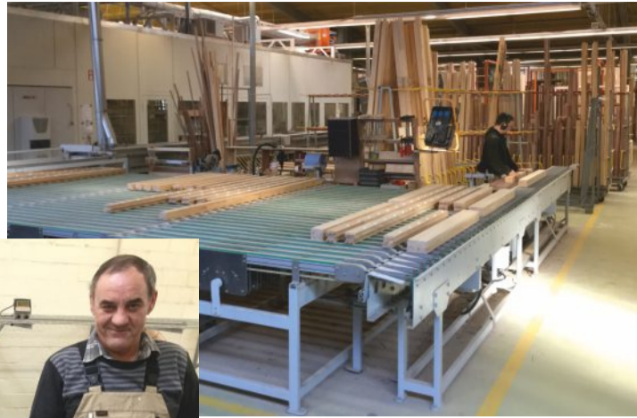
The glazing beads arrive in bar length and are coded according to cross-section. They are cut to length with mitres on the MX-2 to an accuracy of 5/100mm and each end processed for jointing with Hoffmann keys for a secure corner joint.
