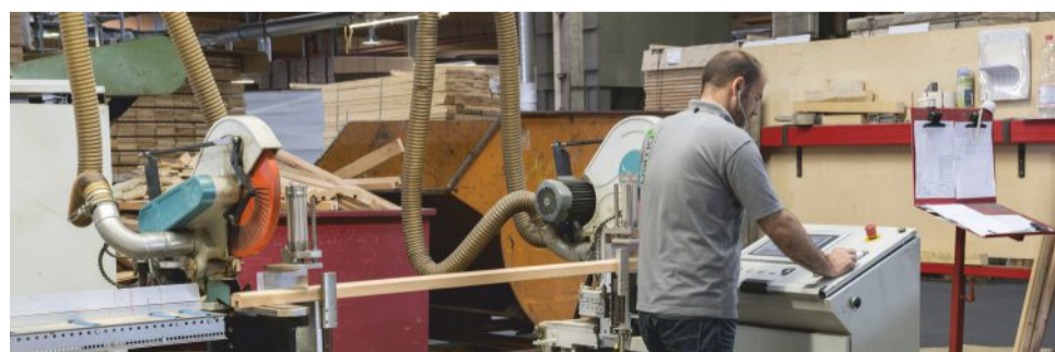
By calling up the article number, length and angle are automatically set
