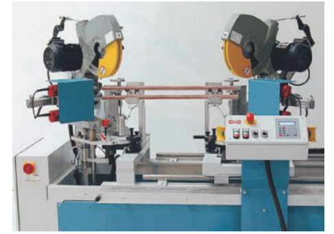
The glazing beads arrive in bar length and are coded according to cross-section. They are cut to length with mitres on the MX-2 to an accuracy of 5/100mm and each end processed for jointing with Hoffmann keys for a secure corner joint.
